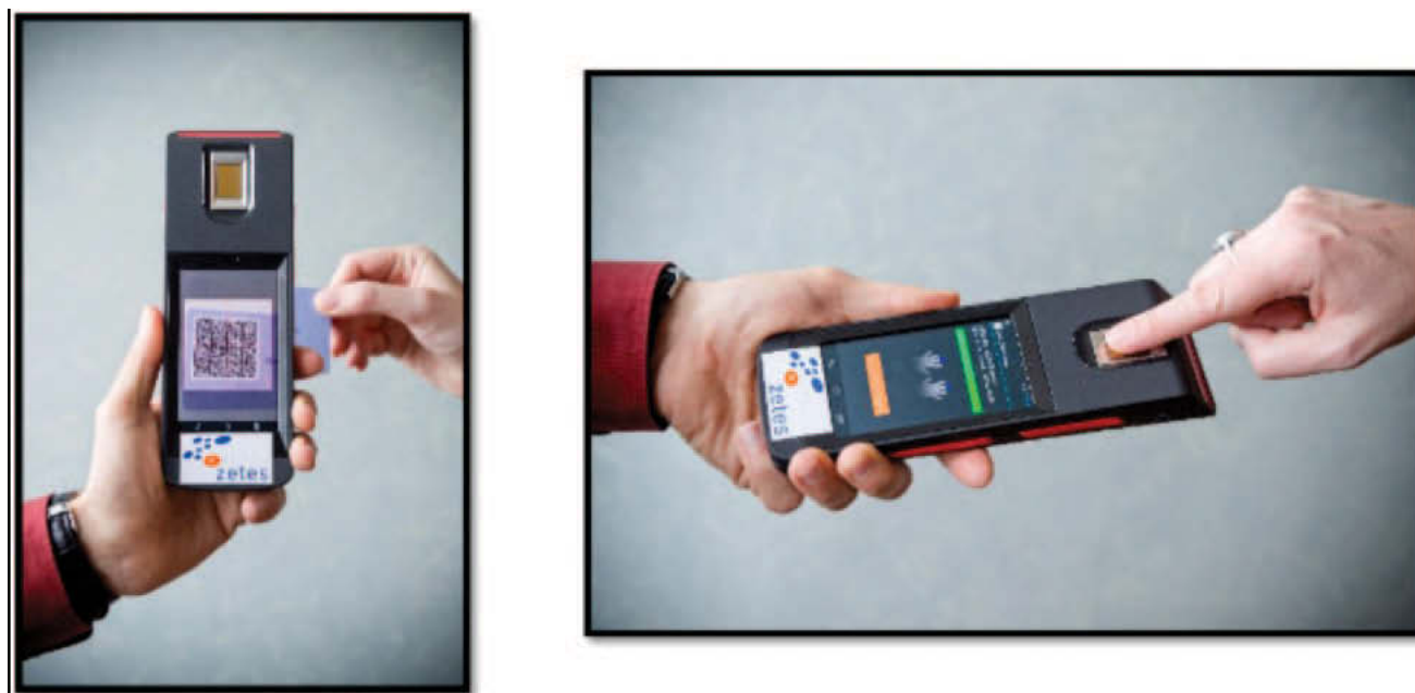
Figure 7: Using Mobile Devices to Authenticate the Identity of the CNAM Card Holder through the Datamatrix 2D Bar Code
